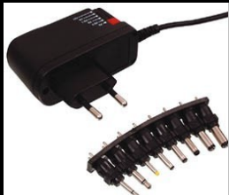
Adapter 3-12 V 1500 mA Input voltage: 110-240 V (AC)/50-60Hz. Switching mode type
