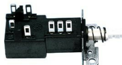
Прекидач 4 / 100 A 250 V 2 pole ON with change over / momentary contact Mounting: 23mm diam. 3.2mm
